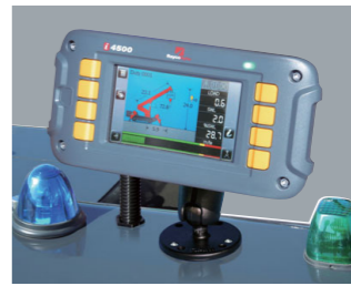
7 Safe load indicator
